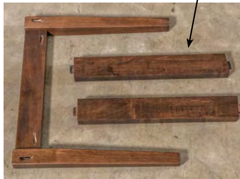
leg assembly glued & pocket-screwed
