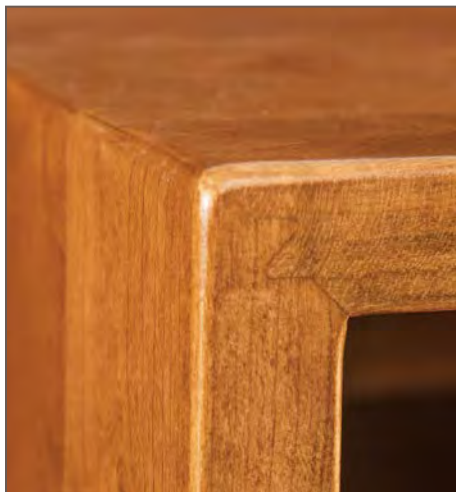
Locking mitered corners
