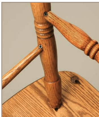
Joined using both screws and glue
