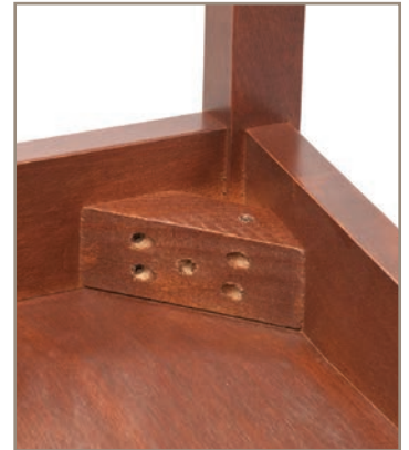
Corner block strengthens corners
