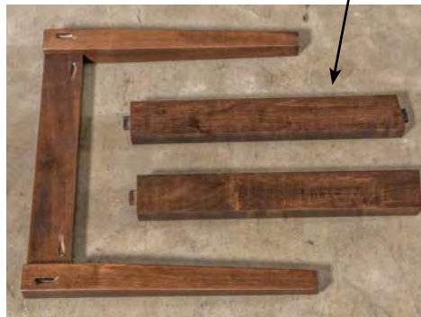
leg assembly glued & pocket-screwed
