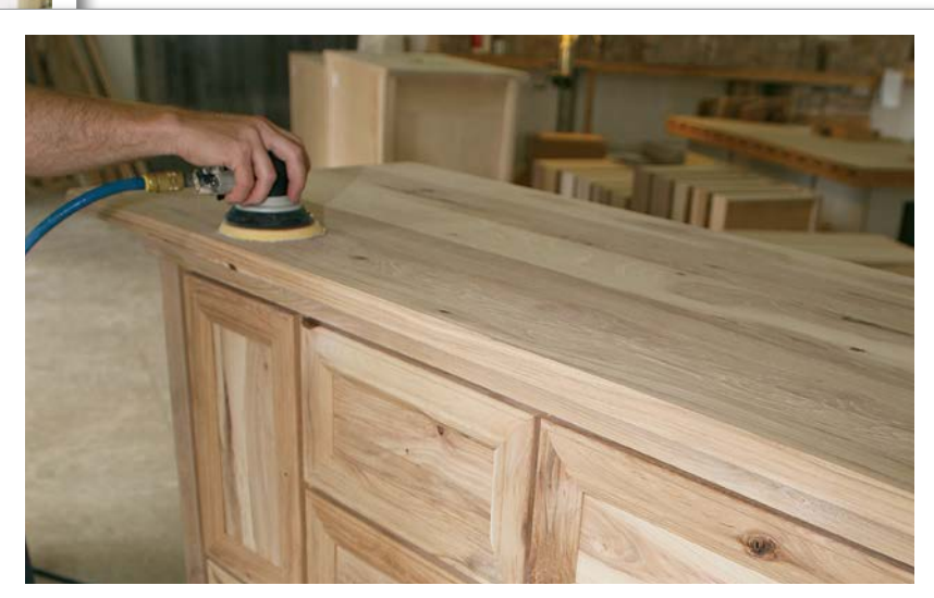
Each piece is hand sanded, preparing it to be finished.
