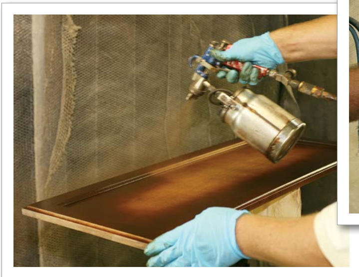
Stain is sprayed then wiped off for an even color tone.
