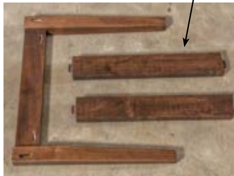
leg assembly glued & pocket-screwed
