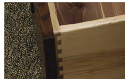
Dovetail joinery is a time-honored technique that connects each board with interlocking pins and tails.
